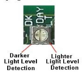
When adjusting the Day/Night Sensor POT you must first set the DIP switches 3 & 4 "Up" when the board is powered down, and then turn the board on. The "Red Control LED" will light up when the detection level detects darkness. You may want to adjust this in the darkest setting you want to run your system at when adjusting this POT. When finished you will need to return DIP switches 3 & 4 back to their original setting.
